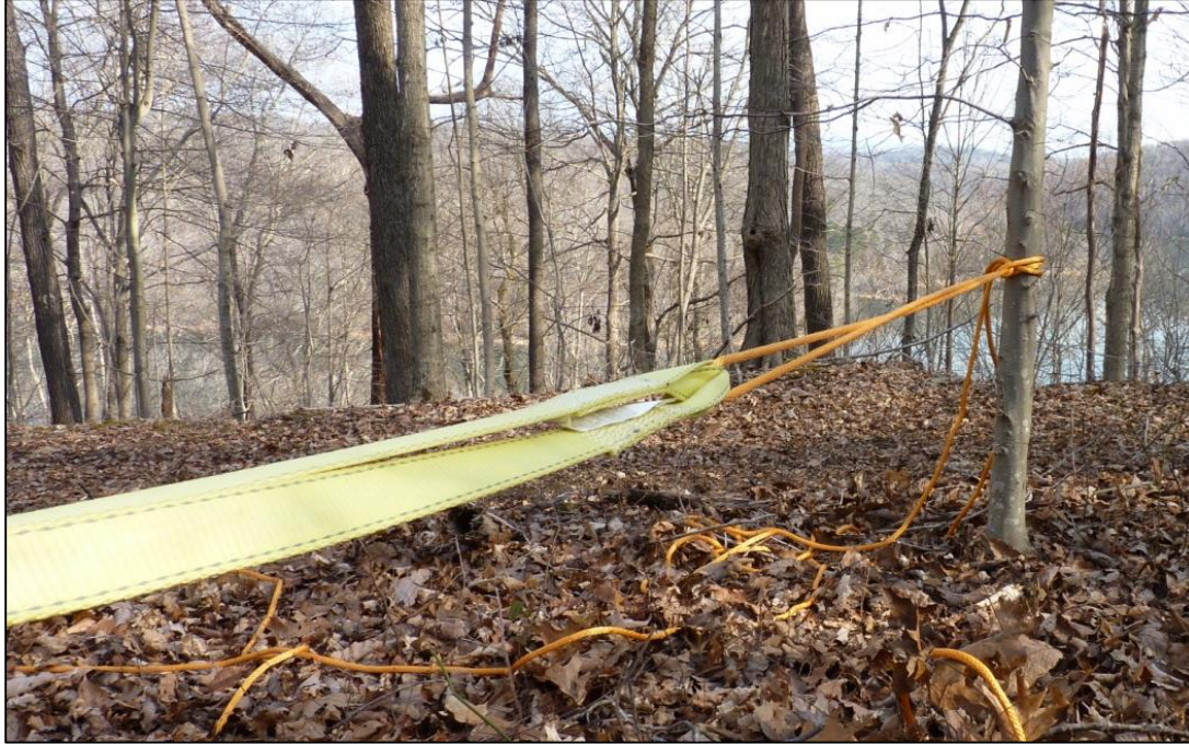
Figure 3.3. Use of a tow strap and rope to remove a stuck borer from a tree (Photograph by Kyle Landolt).
